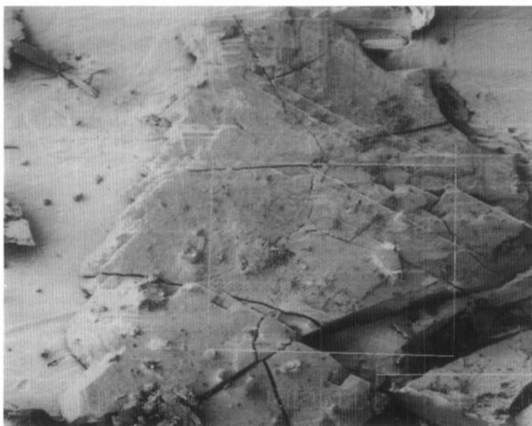
FIG. 4. Secondary electron image of the electrochemically assisted synthesized \text{ZnSiP}_2 (fluorosilicate silicon donor). 3 kV, 100\text{ }\mu\text{m} .
