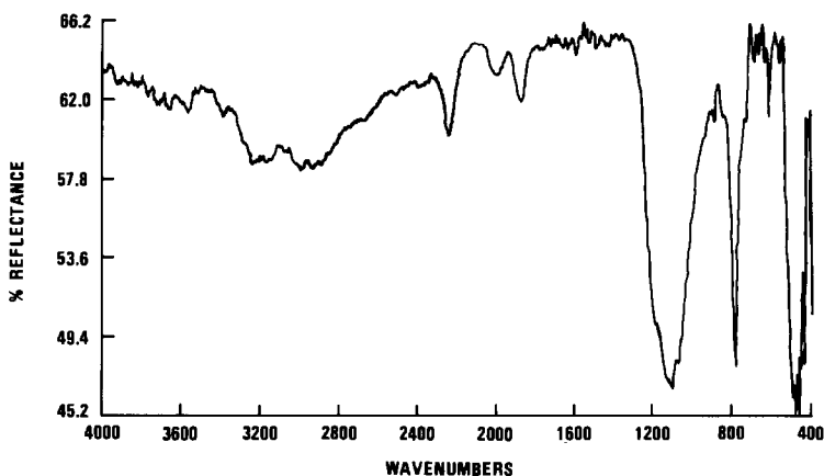
FIG. 3. Diffuse reflectance spectrum of \text{ZnSiP}_2 crystals synthesized by the electrochemically assisted route.
